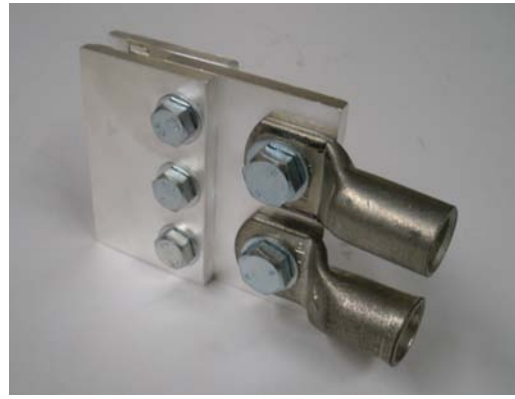
Temporary cable connection onto 6.35mm busbars (approx 2000A)
