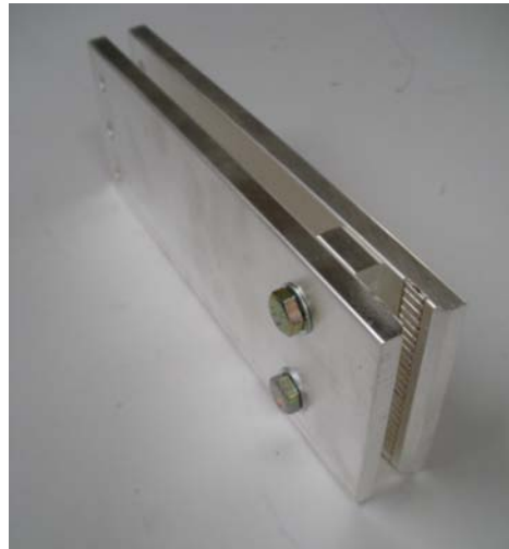
Connection plate for permanent extension of 10mm thick main busbars (approx 3500A)
